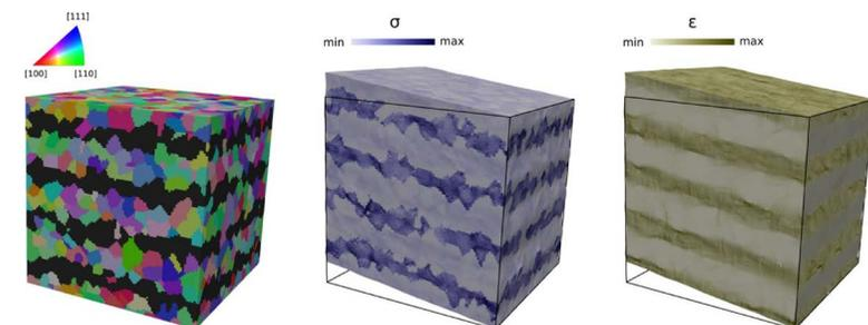
Figure 1. Crystal plasticity simulation of a dual-phase steel: Left: Undeformed microstructure, the ferritic grains are colored according to their crystallographic orientation (inverse pole figure, IPF) and the martensitic phase is shown in black. Middle: equivalent stress at approx. 10% shear deformation. Right: Equivalent strain at approx. 10% shear deformation
